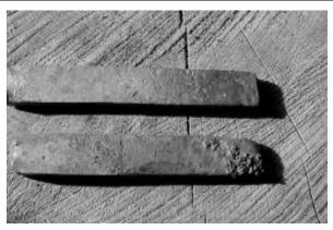
Photo 12: The bottom bar has been burned. The top bar has been burned then slightly up set and reworked – alas, the damage has been done.
