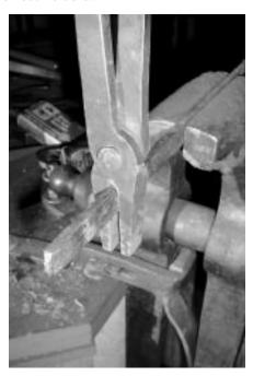
Photo 11: Correcting a twist with a pair of tongs and the bar held in the vise horizontally.
