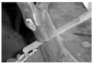
Photo 14: Scraping along a sharp anvil corner to get rid of scale before forging. Use the hammer head to apply downward pressure.
