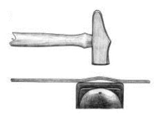
An isolated bend in an otherwise straight bar.
