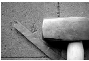
Photo 13: The marks left on the bar came from this poorly dressed hammer face.
